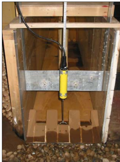
Figure 18. — Deflector and ADV velocity probe installed in Mason Dam stilling basin model.
