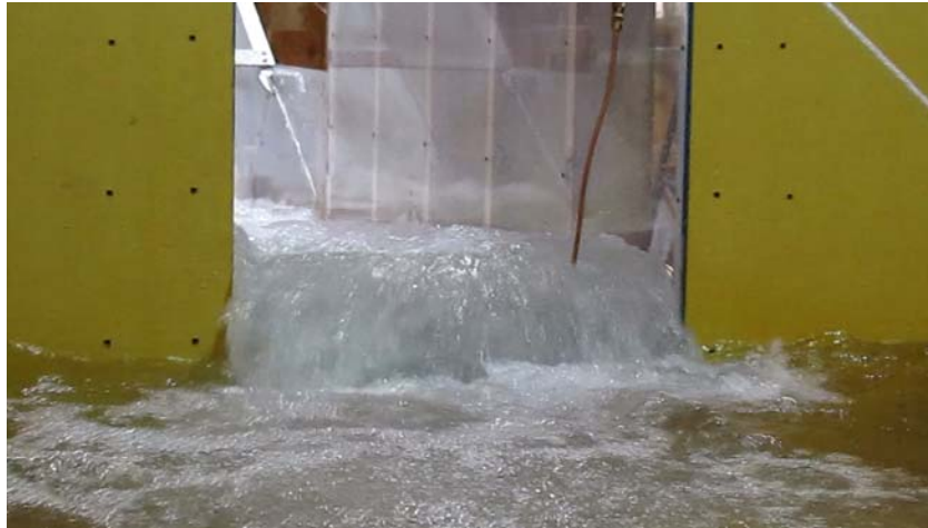
Figure A-112. — Flow over the top of a single deflector at design flow (956 ft 3 /s), with deflector bottom lip located 6.2 ft above basin floor.
