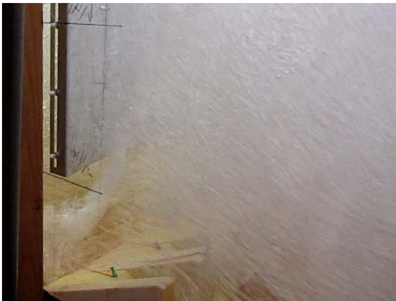
Figure A-10. — Single deflector at design flow (956 ft 3 /s) with deflector bottom edge located 5.1 ft above basin floor.
