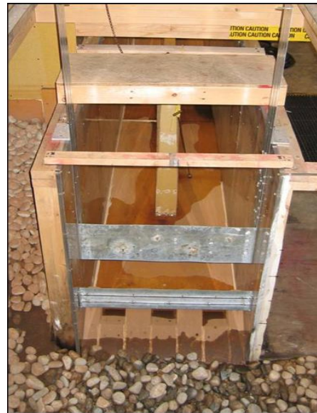
Figure 26. — Mason Dam stilling basin staggered deflector configuration
