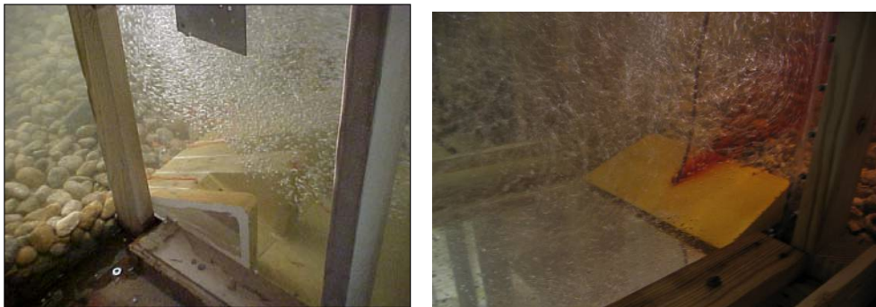
Figure 11. — Strings and dye indicate flow near the bottom is redirected downstream after the deflector is installed in the Mason Dam (L) and Haystack Dam (R) stilling basin models.
