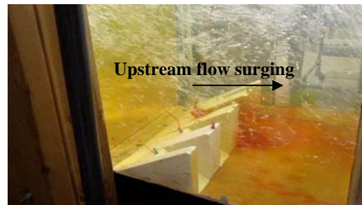
Figure A-5. — Strings and dye indicate currents surging upstream over the basin end sill with potential to carry materials into the stilling basin at flow rates a) 396 \text{ ft}^3/\text{s} , b) 746 \text{ ft}^3/\text{s} , and c) 569 \text{ ft}^3/\text{s} .
