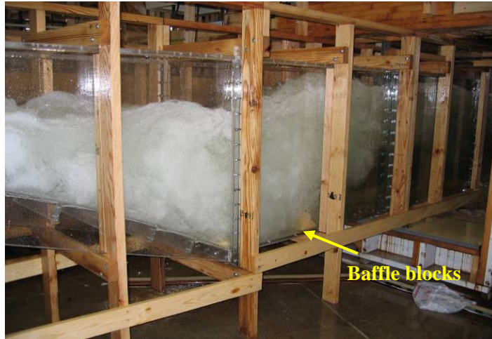
Figure 31. — Baffle blocks help lift jet above basin floor.
