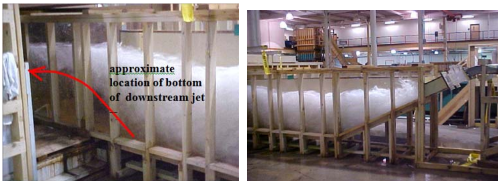
Figure 25. — At lower discharge the jet rises high into the water column (left photo). As discharge is increased the aerated jet travels a longer distance along the basin floor (right photo).
