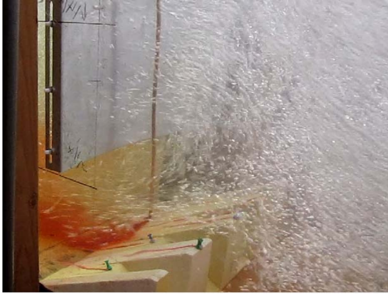
Figure A-10. — Single deflector at 746 ft 3 /s with deflector bottom edge located 5.1 ft above basin floor. Bottom velocities appear to be below the threshold where significant vortex development occurs.
