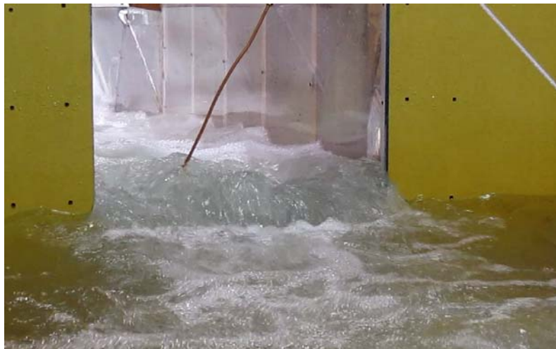
Figure A-123. — Flow over the top of staggered deflectors at design flow (956 ft 3 /s) with the lowest deflector bottom edge located 6.2 ft above basin floor.
