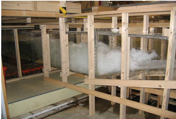
Figure 20. — Choke Canyon stilling basin model operating at 40% gate opening based on maximum reservoir.
