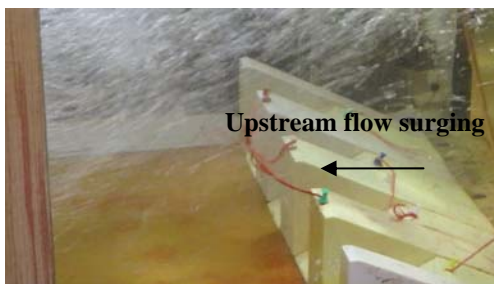
Figure A-5. — Strings and dye indicate currents surging upstream over the basin end sill with potential to carry materials into the stilling basin at flow rates a) 396 \text{ ft}^3/\text{s} , b) 746 \text{ ft}^3/\text{s} , and c) 569 \text{ ft}^3/\text{s} .
