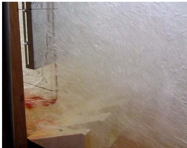
Figure A-9. — Staggered deflector configuration at design flow (956 ft 3 /s) with lowest deflector bottom edge located 6.2 ft above basin floor.
