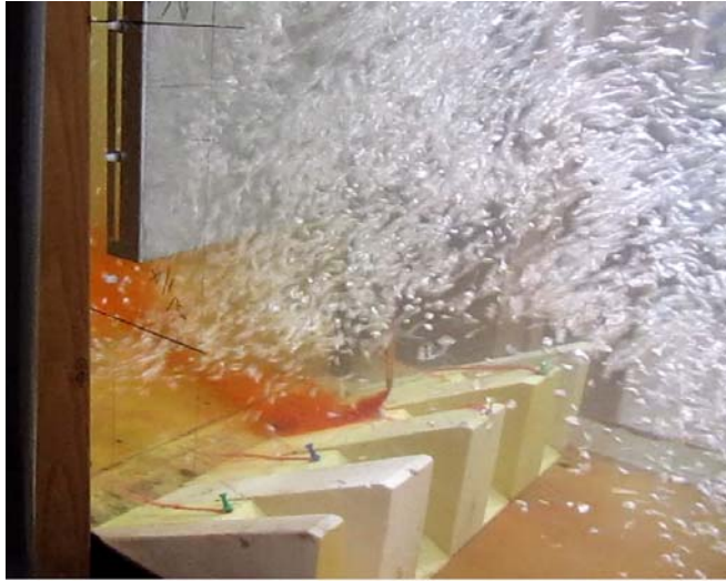
Figure A-8. — Staggered deflector configuration at 396 ft 3 /s, with lowest deflector bottom edge located 6.2 ft. above basin floor.
